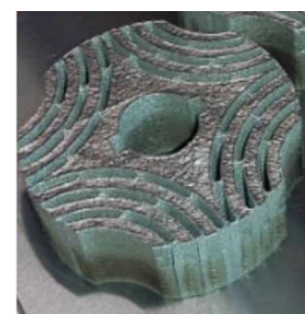
Fig. 2: SynRM-Toror produced by selective laser melting 2
